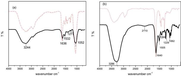
FTIR spectra of (a) Amk@PVP-AqNPs (dotted line) and amikacin (solid line) and (b) Van@PVP-AqNPs (dotted line) and vancomycin (solid line).
