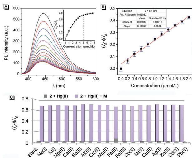
Fig. 6 (A) Fluorescence spectra of **2** upon the addition of Hg(II). Inset: The fluorescence intensity at 445 nm as a function of the Hg(II) concentration. (B) Calibration curve for the emission of **2** with increasing concentrations of Hg(II). (C) Fluorescence intensity at 445 nm in the presence of 0.5 equiv. of different metal ions. Conditions: the concentration of **2** was  $10 \mu\text{mol L}^{-1}$ , 99% water/DMSO (v/v) at pH 7.0 controlled by  $10 \text{ mmol L}^{-1}$  Tris solution.
