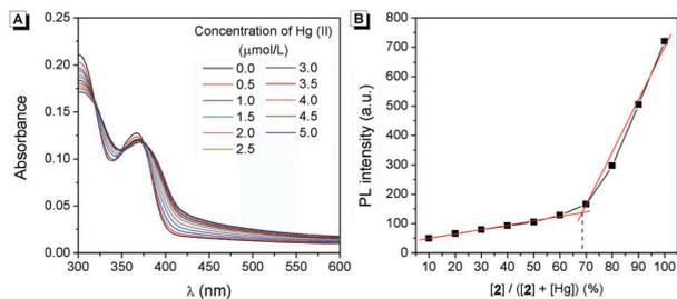
**Fig. 7** (A) Absorption spectra of  $10 \mu\text{mol L}^{-1}$  **2** upon the addition of  $\text{Hg(II)}$ . (B) Job's plot data for evaluating the stoichiometry of the **2-Hg-2** complex. The total concentration of **2** and  $\text{Hg(II)}$  was kept at  $20 \mu\text{mol L}^{-1}$ . 99% water/DMSO (*v/v*) at pH 7.0 controlled by  $10 \text{mmol L}^{-1}$  Tris solution was used. Excitation and emission were performed at 368 nm and 445 nm, respectively.
