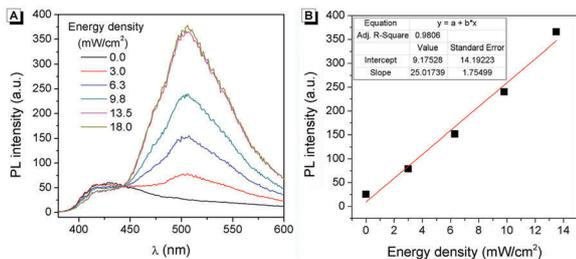
Fig. 4 (A) Fluorescence spectra of  $10 \mu\text{mol L}^{-1}$  of **2** in THF irradiated by 365 nm light with different irradiation intensities for 5 s. (B) Fluorescence intensity at 506 nm as a function of irradiation intensity.
