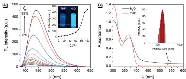
**Fig. 1** (A) Fluorescence emission spectra of  $50 \mu\text{mol L}^{-1}$  **2** in water/THF mixtures with different  $f_w$ . Inset: Fluorescence intensity of **2** at 445 nm as a function of  $f_w$  and fluorescence photograph of **2** in THF and  $\text{H}_2\text{O}$  (99% water/THF (v/v) solution). (B) Absorption spectra of  $50 \mu\text{mol L}^{-1}$  **2** in THF and  $\text{H}_2\text{O}$ . Inset: DLS results of **2** in  $\text{H}_2\text{O}$ .
