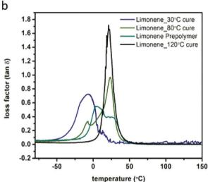
Fig. 4 Representative tensile analysis curves performed at ambient conditions comparing monomer structure (a) and DMA loss factor curves comparing curing conditions of limonene networks (b).
