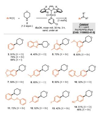
Scheme 1 Aryl halide scope of mechanochemical Buchwald-Hartwig reaction. Reaction conditions: Arylhalide (1 mmol), amine (1.2 mmol), Pd-PEPPSI-iPENT (1 mol%), tBuOK (2 mmol), sand (0.338 g), 15 mL Jar, 1 x 12 g stainless steel ball, 3 h under air in mixer mill. Isolated yields reported
