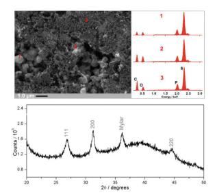
Fig. 3 SEM/EDX analysis and XRD pattern of the as-synthesized  $\rm Li_3PS_4/Li_2S/C$  composite.
