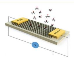
Fig. 5 A schematic design of the flat or patterned MLG-based sensors for E/I/A-containing cancer marker detection. Graphene is placed on a flexible PVC substrate of 25 µm thickness. A two-point measurement concept was used for the in situ electrical characterization of CMinduced graphene electrodes and its selectivity analysis.
