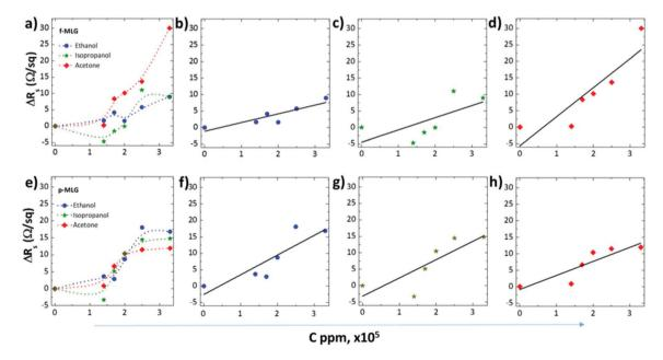
Fig. 4 Sensitivity identification of f-MLG (a) and p-MLG (e) electrodes at various concentrations of cancer marker solutions (ethanol -  $\bullet$ , isopropanol -  $\star$ , and acetone -  $\bullet$ ). Changes in the value of sheet resistance ( $\Delta R_s$ ) for f-MLG (b-d) and p-MLG (f-h) as a function of CM concentration.
