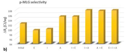
Fig. 6 Selectivity analysis for cancer marker detection by monitoring the sheet resistance value for the three types of organics in various combinations with f-MLG (a) and p-MLG-based (b) electrodes: single solutions of ethanol (E), isopropanol (I), acetone (A); double solutions - E + I, E + A, and A + I; and the triple solution -E + I + A.
