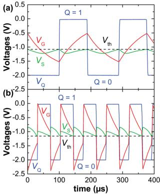
Fig. 2 The measured waveforms in the oscillators in air ambient for  $V_{\rm SS}=-2$  V,  $R_{\rm S}=1.26$  k $\Omega$ , and C=1 nF. (a) The waveforms in the parabolic oscillator with R=85 k $\Omega$  resulting in the oscillation frequency  $f_{\rm osc}=5.3$  kHz and duty cycle D=46%. (b) The waveforms in the bow tie oscillator with R=57 k $\Omega$ ,  $f_{\rm osc}=13.8$  kHz, and D=55%.
