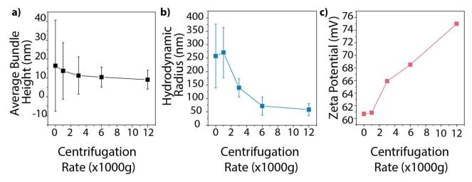
Fig. 8 Tracking the impact of centrifugation rate on the (a) average BNNT bundle height measured using AFM, (b) hydrodynamic radius, and (c) zeta potential of BNNTs dispersed in CTAB. Increasing centrifugation rate produces smaller and more uniform dispersions with increased stability.
