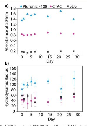
Fig. 7 BNNT dispersions in SDS, CTAC, and Pluronic F108 tracked over one month by (a) UV absorbance and (b) DLS. Both measurements show no significant changes over time confirming that the dispersions are stable.
