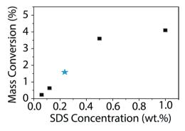
Fig. 6 Mass conversion (%) of BNNTs as a function of SDS concentration. The initial nanotube concentration is  $1 \text{ mg mL}^{-1}$ . The published CMC for SDS is 0.236 wt% (ref. 53) and is denoted with a blue star. BNNT mass conversion quickly increases once the concentration of SDS is above the CMC with a maximum of approximately 4% conversion in 1 wt% SDS.
