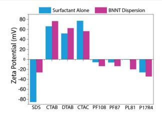
Fig. 3 Zeta potentials measured for each surfactant and surfactant-BNNT dispersion. The zeta potential reveals the degree of electrostatic repulsion between nearby particles and is an indicator of dispersion stability. The chart reveals a similar trend, among ionic surfactants, to that seen for their mass conversion
