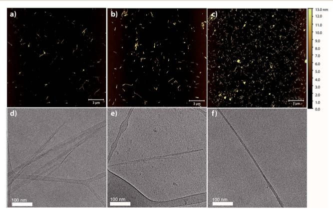
Fig. 4 AFM and cryo-TEM images of BNNT dispersions in SDS (a, d), CTAB (b, e), and Pluronic F108 (c, f). The images reveal that the BNNTs in our dispersions are primarily individualized or in small bundles.
