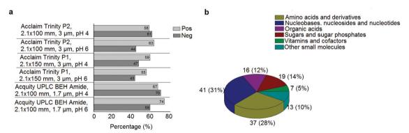
Fig. 2 (a) Percentage of metabolites found in a 10 μM multicomponent standard with the different HILIC columns at pH 4 and pH 6 in positive and negative mode. When combining positive and negative mode, the UPLC BEH Amide column at pH 4 showed the highest coverage. (b) The number of metabolites and their classes (combining positive and negative mode) as found in a  $10 \,\mu\text{M}$  multicomponent standard of > 130 metabolites with the UPLC BEH Amide column at pH 4.
