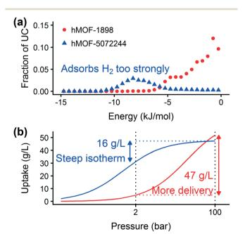
Fig. 2 (a) Case study of two MOFs, hMOF-1898 and hMOF-5072244, with different pore energetics. (b) Although the MOFs have similar saturation loadings, their deliverable capacity is considerably different due to the amount of hydrogen remaining in the tank at low pressure. Dashed lines designate the delivery and storage pressures of 2 bar and 100 bar, respectively. The x-axis is plotted on a log scale.
