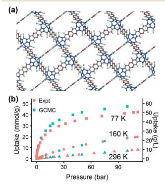
Fig. 8 Applying the trained hMOF model for screening the CCDC MOF database. (a) Structure and (b) hydrogen adsorption isotherm for MFU-4l, a high-performing MOF selected for experimental validation. Red symbols are isotherm points from experiment and blue points are from GCMC simulations at 77 K (squares), 160 K (circles), and 296 K (triangles).
