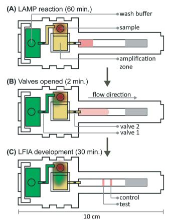
Fig. 4 Schematic of fluid travel through microRAAD. (A) The wash buffer (green) is constrained from flowing to the amplification zone and the sample (red blood cells and yellow plasma) is constrained from flowing to the LFIA by closed valves. (B) Upon thermally actuating the valves, wash buffer is released to the amplification zone and the RT-LAMP products migrate to the LFIA for (C) test band development.
