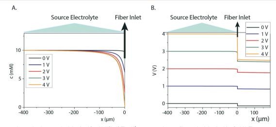
Fig. 3 Concentration and voltage at the inlet for 10 mM KCl. A) The  $K^+$  concentration profiles at the inlet for V = 0-4 V. The curves for 3 V and 4 V are nearly identical. B) Voltage profiles for V = 0-4 V. For lower voltages the voltage drop at the CEM is quite small, while at limiting current conditions (V = 3 V and 4 V) additionally applied voltage is dropped at the interface (x: distance from fiber inlet).
