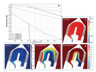
Fig. 2 COMSOL simulations to determine (A) the recovery rate of the  $\mu$ PPPS probe tip as a function of flow rate (*x*-axis) and outlet pressure (legend). Velocity profile (m s<sup>-1</sup>) (B) and concentration profile (C) using 50 nL min<sup>-1</sup> and -10 kPa outlet pressure. Pressure distribution (E) and concentration profile (D) for a flow rate of 50 nL min<sup>-1</sup> and -80 kPa outlet pressure. Note that the pressure outside the probe is set to 1 bar (101.32 kPa).
