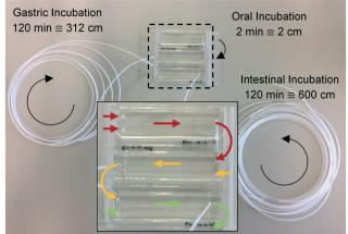
Fig. 3 Photograph of the three micromixers, coupled in series, for the digestion of lactoferrin. The arrows represent the flow direction in each of the modules (red: mouth; yellow: stomach; green: intestine). Loops of tubing of 2, 312 and 600 cm were used for incubation after each stage, corresponding to 2, 120 and 120 min incubation time. All inlet tubings have been removed for clarity.
