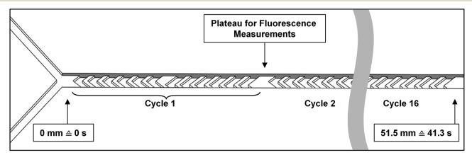
Fig. 2 Diagram of a micromixer channel, containing herringbone-shaped grooves in its surface. Two inlet channels are visible at the left. The channel is just over 50 mm long, and contains 16 cycles of 12 grooves each. Between cycles, a plateau is incorporated to allow for a 300 × 100 μm measurement region. At a total flow rate of 2.0 μL min<sup>-1</sup>, as used in the enzyme kinetics experiments, 51.5 mm channel length corresponds to a residence time of 41.3 s.
