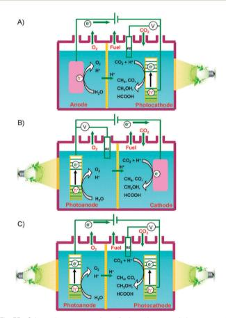
Fig. 35 Schematic representation of photoelectrocatalytic reactors in two-compartment cells separated by proton-exchange membranes. CO<sub>2</sub>RR and water oxidation occur over the cathode and the anode sides, respectively. The alternative or simultaneous utilization of photocatalysts under light irradiation on the cathode and anode side is represented in each case. Reprinted with permission from ref. 539. Copyright The Royal Society of Chemistry 2016.
