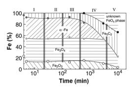
Fig. 11 Iron-phase composition as a function of time during the Fischer-Tropsch synthesis under CO<sub>2</sub> atmosphere, determined by Mössbauer spectroscopy. Data collected with a Cu-K-doped Fe-Al catalyst at 250 °C, 1 MPa, and  $H_2/CO_2 = 3$ . Reproduced with permission from ref. 138. Copyright 2003 Springer Nature.
