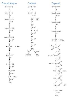
Fig. 27 Proposed formaldehyde, carbine, and glyoxal pathways for the CO<sub>2</sub>RR to produce CH<sub>4</sub>. Readapted with permission from ref. 404. Copyright 2013 John Wiley and Sons.
