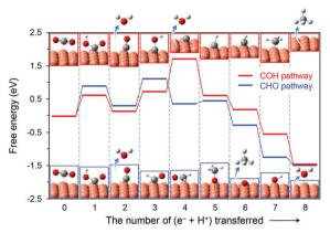
Fig. 19 Multi-step conversion of CO<sub>2</sub> to CH<sub>4</sub>, indicating the calculated free energies (at zero external bias) for alternative pathways considering the formation of CHO\* (blue) and COH\* (red) intermediates. 264,265 Molecular species at each step are identified. Reprinted with permission from ref. 263. Copyright 2017 American Chemical Society.
