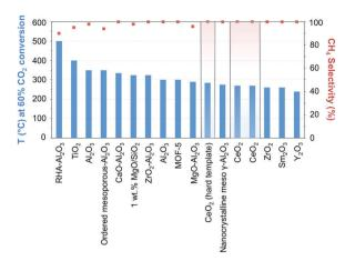
Fig. 7 Performance of Ni-based catalysts in t-CO<sub>2</sub>RR to CH<sub>4</sub>, tentatively compared on the basis of the temperature necessary to achieve ca. 60% CO<sub>2</sub> conversion. The highlighted results indicate the overall superior performance of Ni/CeO2 catalysts in the literature. Further details and respective references have been conveniently summarized in Table 1.
