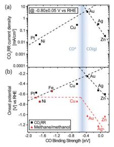
Fig. 16 (a) Volcano plot of partial current density for the e-CO<sub>2</sub>RR assessed at -0.8 V vs. CO binding strength. (b) Distinct onset potentials plotted vs. CO binding energy for the overall e-CO2RR, and for methane/ methanol production. Dashed lines serve as a guide. Reprinted with permission from ref. 245. Copyright 2014 American Chemical Society.
