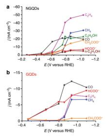
Fig. 23 Partial current densities of emerging CO<sub>2</sub>RR products as a function of the applied potential over (a) N-doped graphene quantum dots (NGQDs) and (b) GQDs cathodes. Adapted with permission from ref. 357. Copyright 2016 Springer Nature.
