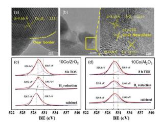
Fig. 8 (a) TEM images of calcined catalyst precursors Co<sub>3</sub>O<sub>4</sub>/ZrO<sub>2</sub> and (b) the corresponding reduced catalyst  $\text{Co/ZrO}_2$ . (c) and (d) are the O 1s XPS spectra for the  $Co/ZrO_2$  and  $Al/Al_2O_3$  catalysts calcined, following  $H_2$ reduction, and after 8 h on stream. Readapted with permission from ref. 121. Copyright 2018 Elsevier B.V.
