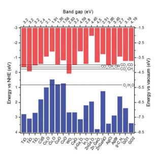
Fig. 25 Band edge positions for selected photocatalysts in the p-CO<sub>2</sub>RR. Results summarized by Jaroniec and colleagues were based on references listed in the review. Particularly, for the listed TiO<sub>2</sub>, Cu<sub>2</sub>O, CuO, and GO, the reader is referred to the published works.  $^{397-402}$  Reproduced with permission from ref. 392. Copyright The Royal Society of Chemistry 2015.
