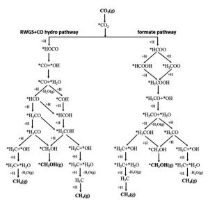
Fig. 3 Schematic representation of the proposed RWGS + CO-hydro and formate mechanistic pathways in the selective t-CO2RR to methane. Adapted with permission from ref. 44. Copyright The Royal Society of Chemistry 2016
