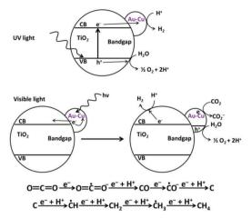
Fig. 32 Schematic representation of the proposed mechanism under UV and visible light for Au-Cu alloy NPs decorated on TiO2 as photocatalysts, to rationalize the influence of the irradiation wavelength range on the product distribution. A proposed route for CO2RR to CH4 in water is represented and in accordance with the carbine mechanism given in Fig. 27. Reprinted with permission from ref. 407. Copyright 2014 American Chemical Society.
