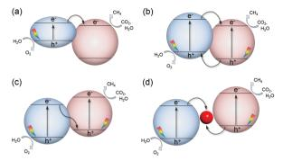
Fig. 28 Schematic representation of formed heterojunctions in the p-CO<sub>2</sub>RR. (a) Sensitization, (b) staggered type heterojunctions, and Z-scheme systems (c) in the absence of a mediator or (d) in the presence of conductive solid mediators (e.g. Au nanoparticles).
