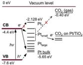
Fig. 30 Schematic diagram of the p-CO<sub>2</sub>RR in the presence of Pt-TiO<sub>2</sub> nanostructured films with a remarkable  $CH_4$  production rate (1361  $\mu$ mol g<sup>-1</sup> h<sup>-1</sup>). Photogenerated electrons are proposed to move fast inside the highly oriented TiO<sub>2</sub> single crystals, flowing to the Pt deposits where the redox reaction occurs to convert CO2 into CH4. Readapted with permission from ref. 397. Copyright 2017 American Chemical Society.
