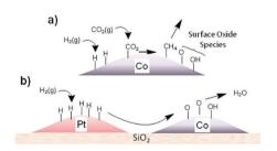
Fig. 9 (a) Schematic representation of the production of surface oxide species during CO<sub>2</sub> methanation and (b) transfer of adsorbed hydrogen from Pt to Co via a spillover mechanism to re-reduce the cobalt oxide surface, releasing water. Reprinted with permission from ref. 128. Copyright 2014 American Chemical Society
