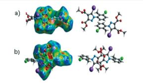
Fig. 9 The presence of  $\pi \cdots \pi$  (a) and CO $\cdots \pi$  (b) interactions predicted by the Hirshfeld surface (shape index). Coloured adjacent red and blue patches present regions of complementarity between two adjacent molecules revealing the presence of such interactions.
