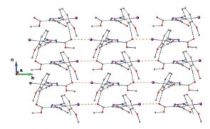
Fig. 5 Two-dimensional supramolecular layer in the crystal structure of 2 viewed along the a-axis. H-atoms not involved in hydrogen bonding are omitted for clarity. The CH···O hydrogen bonds and the short I···O intermolecular contacts are shown in black and orange dashed lines, respectively.
