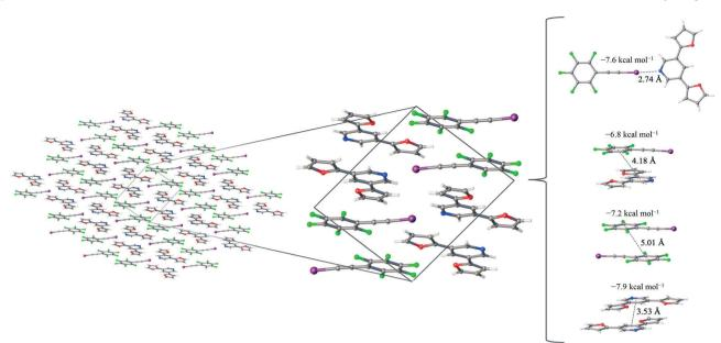
Fig. 2 The  $F_5BAl$ -PyrFur<sub>2</sub> co-crystal, a zoomed in picture of the unit cell which shows the presence of non-covalent interactions as well as the pair-wise contacts with the largest interaction energies labeled with the corresponding distance (in Å) and the average interaction energy (in kcal mol<sup>-1</sup>).
