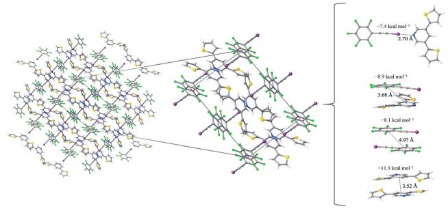
Fig. 3 The  $F_5BAl$ -PyrThio<sub>2</sub> co-crystal, a zoomed in picture of the unit cell which shows the presence of non-covalent interactions as well as the pair-wise contacts with the largest interaction energies labeled with the corresponding distance (in Å) and the average interaction energy (in kcal mol<sup>-1</sup>).
