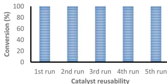
Fig. 1 Recyclability of the complex **2** for the coupling reaction of CO<sub>2</sub> with epichlorohydrin under optimal reaction conditions.
