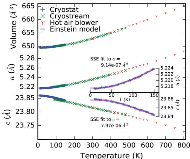
**Fig. 3** Lattice parameters of the  $I4_1/acd$  phase of  $\text{Ca}_2\text{GeO}_4$  as a function of temperature. The temperature devices used for different measurements are indicated in the legend. Inset: The single Einstein mode model plotted against the low temperature data to which it was fitted. Sum of the squared error (SSE) measures of fit shown for each lattice parameter.
