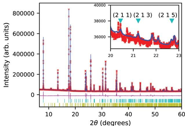
Fig. 2 Rietveld fit to 300 K high resolution X-ray powder diffraction data of  $\text{Ca}_2\text{GeO}_4$  collected at  $\lambda = 0.82661 \text{ \AA}$ . Upper tick marks (cyan) indicate allowed reflections for the main  $I4_1/acd$  phase and lower tick marks (yellow) indicate those associated with the olivine impurity phase. Inset: Superstructure peaks indexed with respect to the  $I4_1/acd$  cell and impurity peaks from the olivine phase that significantly convolute this region.
