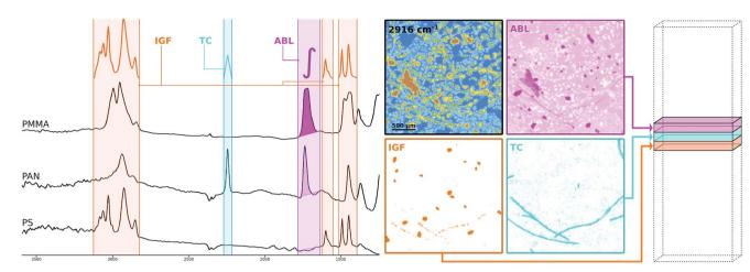
Fig. 2 Descriptor images generated using the ABL, TC and IGF descriptors. The spectra (left) correspond to three types of common polymers. By using the stated spectral descriptors on certain ranges of the hypercube the corresponding descriptor images (middle) can be computed which are then reassembled as a descriptor cube of reduced dimensionality and improved data quality (right).
