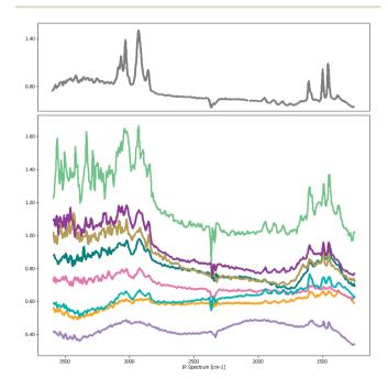
Fig. 1 Polystyrene spectra of varying quality sampled at the center of a particle (upper chart) and at particle edges (lower chart). As particle sizes can be as low as 10  $\mu$ m Mie scattering distorts the baselines of the spectra.
