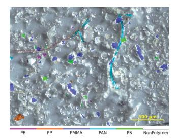
Fig. 5 Zoomed-in overlay of the classification result obtained from the 'Microplastic'† (ref. 31) dataset. The NonPolymer class is transparent so that the underlying image is visible.
