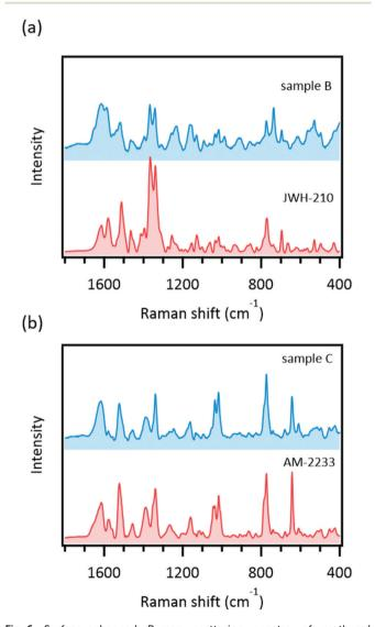
Fig. 6 Surface-enhanced Raman scattering spectra of methanol extracts of sample B and sample C (in blue). Corresponding spectra of standard solutions are also shown (in red). These spectra were obtained by using a Raman microspectrometer with 1-5 s exposure time.
