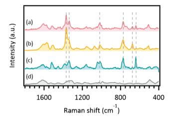
Fig. 3 Surface-enhanced Raman scattering spectra of a real herbal high. (a) Spectrum obtained from sample A (Table 2), (b) standard spectrum of AM-1220, (c) standard spectrum of AM-2233, and (d) background spectrum. Dashed lines indicate peaks that coincide in the sample and standard spectra. Exposure was 1 s, 100 frames.
