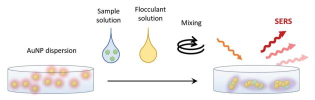
Fig. 1 Schematic of the present SERS experimental system using gold nanoparticle (AuNP) co-aggregation in a wet system.
