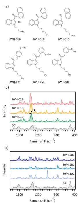
Fig. 2 Measurement of the surface-enhanced Raman scattering spectra of standard solutions. (a) Chemical structures of examined synthetic cannabinoids, (b) spectra of methylene positional isomers, and (c) spectra of methoxy positional isomers. BG indicates the background measurement. Exposure was 1 s, 100 frames. Arrow heads indicate the peaks useful for discrimination.
