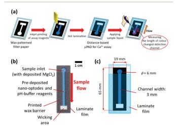
Fig. 1 (a) Schematic procedure of device fabrication by printing technology and Ca<sup>2+</sup> assay with a Ca<sup>2+</sup>-selective distance-based μPAD; (b) design of distance-based μPAD for nano-optode based Ca<sup>2+</sup> detection, and (c) corresponding dimensions representing the settings in the PowerPoint graphic software.
