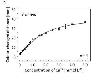
Fig. 3 (a) Scanned images of colour-developed μPADs after application of the corresponding  $Ca^{2+}$  solutions of various concentrations (30  $\mu L$  of aqueous CaCl<sub>2</sub>); (b) software-assisted response curve of a µPAD-based Ca<sup>2+</sup> assay; the response curve represented by the solid line was 165
