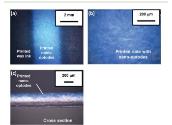
**Fig. 2** Microscope images of nano-optode filter paper substrates: (a) nano-optode modified paper surface of the flow channel; (b) scale-up of the nano-optode modified paper surface; and (c) cross section of nano-optode modified paper.
