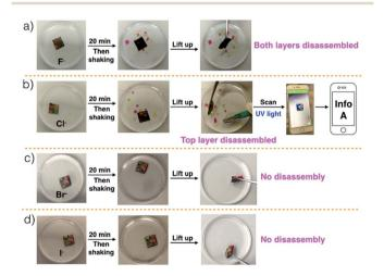
Fig. 4 Photographs of the double layer construct made up from Code B and Code A before and after immersion into chloroform solutions containing various anion salts (a) TBAF, (b) TBACI, (c) TBABr, and (d) TBAI for 20 min. The same concentration (20 mM) and volume (20 mL) were used for all experiments. The size of the substrate is 2.5 cm  $\times$  2.5 cm.
