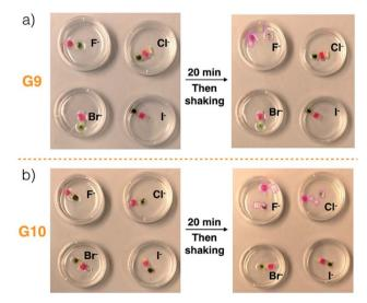
Fig. 3 Photographs of (a) G9 and (b) G10 before and after immersion into chloroform solutions containing various tetrabutylammonium halide anion salts (viz. TBAF, TBACI, TBABr, and TBAI) for 20 min. The same concentrations (20 mM) and volumes (20 mL) were used in all cases. The size scale for constructs G9 and G10 is provided in Fig. 1. Disassembled gel blocks are shown using boxes.
