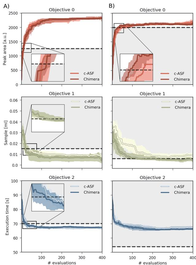
**Fig. 5** Achieved objective function values for multi-objective optimization runs on a virtual robot model obtained with Phoenix on Chimera and c-ASF averaged over 50 individual runs. The goal of the optimization runs is to maximize the HPLC response, minimize the sample volume and minimize the execution time beyond the set bounds, indicated with black dashed lines.
