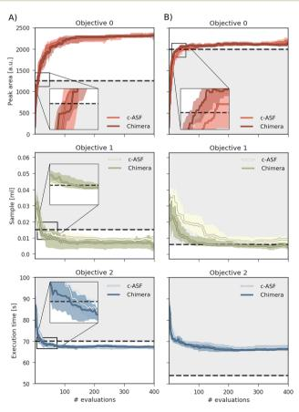
Fig. 5 Achieved objective function values for multi-objective optimization runs on a virtual robot model obtained with Phoenics on Chimera and c-ASF averaged over 50 individual runs. The goal of the optimization runs is to maximize the HPLC response, minimize the sample volume and minimize the execution time beyond the set bounds, indicated with black dashed lines.
