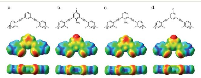
Fig. 4 ChemDraw and ESP maps of G1XBme<sup>2+</sup> (a), G2XBme<sup>2+</sup> (b), G2XBme<sup>2+</sup> with no fluorine (c) and G2XBme<sup>2+</sup> with no amine (d). All ESP maps are displayed on the same scale. Electron-deficient regions are blue and electron-rich regions are red.
