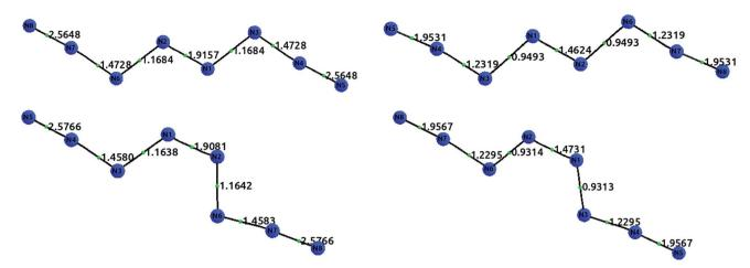
Fig. 6 Optimized structures with delocalization indices displayed for the isomers EEE (top) and EZE (bottom) of the  $N_8$  molecule. The left diagrams show the HF values, and the right diagrams the CCSD values.
