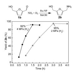
Fig. 5 Time courses of reductive amination of 5-hydroxymethylfurfural (1b) over Ru-NP. Reaction conditions: catalyst (0.2 mg), 1b (0.5 mmol), MeOH (5 mL), NH $_3$  (8 mmol), and H $_2$  (2 and 4 MPa), 363 K
