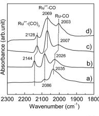
Fig. 4 Difference DRIFT spectra for adsorption of CO onto (a) Ru-NP, (b) Ru/Nb $_2$ O $_5$ , (c) Ru/SiO $_2$  and (d) Ru-HCP samples at 103 K.
