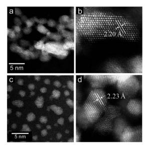
Fig. 1 (a) HAADF-STEM and (b) high magnification HAADF-STEM images of Ru-NPs prepared from 10 wt% Ru-deposited  $Ca(NH_2)_2$ . (c) HAADF-STEM and (d) high magnification HAADF-STEM images of 10 wt% Ru/Ca(NH<sub>2</sub>)<sub>2</sub>.
