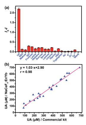
Fig. 5 (a) Quenching effect of NIR-II signal at 1530 nm of the NCs/uricase solution under 980 nm excitation after incubation with 1 mM UA or other different analytes. Error bars represent the standard deviations of triplicate experiments. (b) Correlation between NCs-based assay and commercial kit for the detection of UA in 24 human serum samples, which were kindly provided by Fujian Provincial Cancer Hospital, Fuzhou, China. Each data point represents the mean of triplicate experiments.
