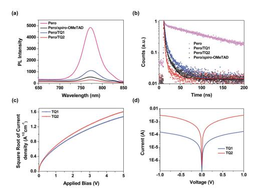
Fig. 5 (a) Steady-state PL spectra of the MAPbl₃ perovskite films with or without capping different HTMs. (b) Time resolved photoluminescence decay at 770 nm for the pristine perovskite film and the perovskite films capping different HTMs. (c) The space-charge-limited-current (SCLC) measurements of hole only devices with the configuration of ITO/PEDOT:PSS/HTM/Au. (d) The conductivity measurements of TQ1 and TQ2.
