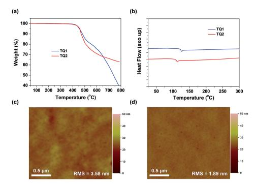
Fig. 3 (a) Thermogravimetric analysis of TQ1 and TQ2 measured with a heating rate of 10 °C min<sup>-1</sup>. (b) The second DSC heating traces of HTMs previously heated and cooled with a scan rate of 10 °C min<sup>-1</sup> under a nitrogen atmosphere. (c and d) Top-view AFM images of TQ1 and TQ2 thin films deposited on the perovskite layer, respectively.
