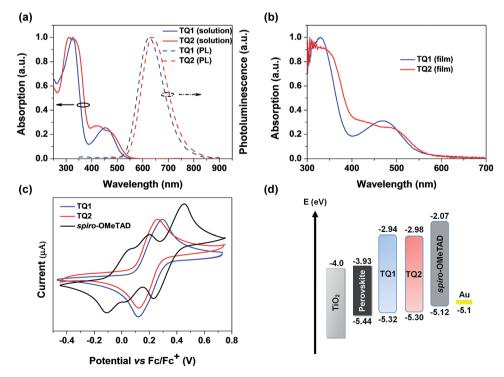
Fig. 2 (a) Absorption and emission spectra of TQ1 and TQ2 in CH<sub>2</sub>Cl<sub>2</sub>. (b) Absorption spectra of TQ1 and TQ2 in the thin film state. (c) CV spectra of TQ1, TQ2 and spiro-OMeTAD. (d) Energy-level diagram of perovskite solar cells with different HTMs (energy levels of the perovskite, TiO2 and Au are taken from ref. 8).
