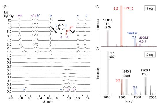
Fig. 5 (a)  $^{1}$ H NMR titration spectra of CS (1 mM) with the addition of  $H_{2}PO_{4}^{-}$  in CDCl<sub>3</sub>. (b) ESI-MS of CS (1 mM) with 1 eq. TBAH<sub>2</sub>PO<sub>4</sub> and (c) 2 eq. TBAH<sub>2</sub>PO<sub>4</sub> (20 V, 50 °C source).
