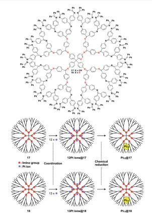
Fig. 5 Dendrimer-based 0D scaffolds for the assembly of a fixed number of metal ions. When Pt ions are accumulated in the interior and subsequently reduced, Pt clusters are formed.
