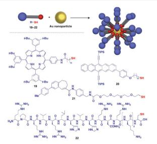
Fig. 6 Schematic structure of an AuNP-based 0D scaffold and examples of functional molecular units (blue) assembled with the scaffold. TIPS = triisopropylsilyl.
