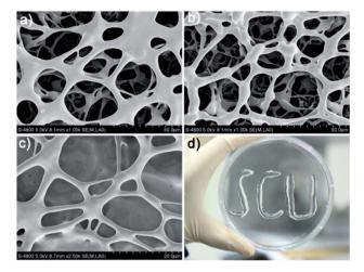
Fig. 1 SEM images of the coordination polymer hydrogels formed by  $AgNO_3$  with (a) 1a, (b) 1b, and (c) 1c. (d) An image of the characters "SCU" injected by the coordination polymer hydrogel formed by Ag/1c with a 3 mL glass syringe.
