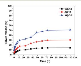
Fig. 3 Cumulative release profiles of silver from the coordination polymers Ag/1a-c at 37 °C in 10.0 mM PBS at pH 7.4.
