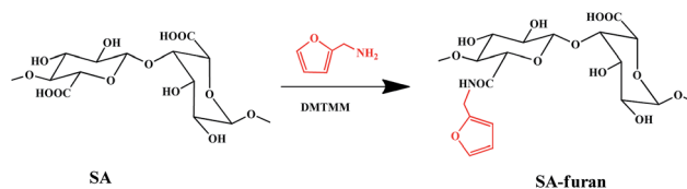
Scheme 1 Synthesis steps of SA-furan.
