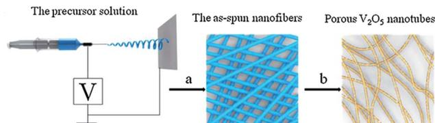
Fig. 5 Electrospinning preparation of porous  $V_2O_5$  nanotubes: (a) electrospinning process; (b) annealing process.<sup>76</sup>
