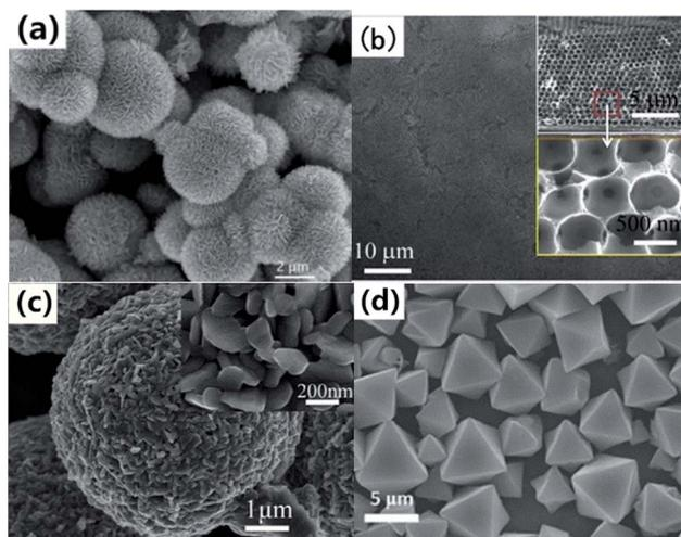
Fig. 10 (a) SEM images of  $V_2O_5$  precursor.<sup>96</sup> (b) Multilayer  $V_2O_5$  hollow sphere arrays (cross-sectional SEM images in inset).<sup>99</sup> (c) SEM images of the  $V_2O_5$  product synthesized by annealing the corresponding VEG precursors in air.<sup>101</sup> (d) FESEM images of ammonium vanadium oxide octahedrons.<sup>102</sup>
