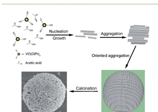
Fig. 11 Schematic of the formation of 3D porous  $V_2O_5$  hierarchical microspheres.<sup>103</sup>
