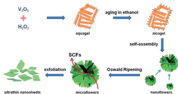
Fig. 8 Schematic illustration of the procedure for fabricating the ultrathin vanadium oxide nanosheets.<sup>87</sup>
