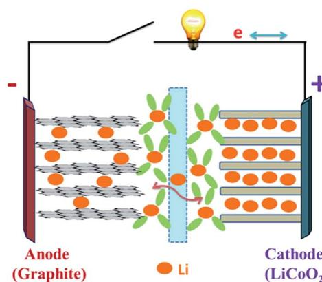
Fig. 1 Schematic of a lithium-ion battery during the charge/discharge process.<sup>25</sup>
