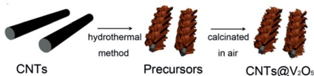
Fig. 13 Schematic of the synthesis process for CNTs@ $V_2O_5$ .<sup>127</sup>
