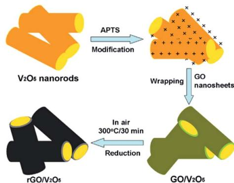
Fig. 14 Schematic of the fabrication of rGO enwrapped  $V_2O_5$  nanorods.<sup>140</sup>
