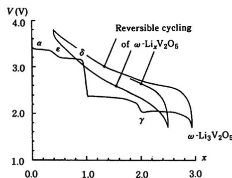
Fig. 2 Various phases associated with the electrochemical intercalation of lithium into V<sub>2</sub>O<sub>5</sub>.<sup>40</sup>
