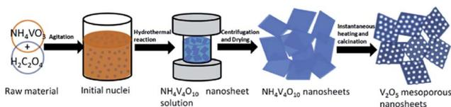
Fig. 9 Schematic of the synthesis route of  $V_2O_5$  mesoporous nanosheets in this work.<sup>89</sup>
