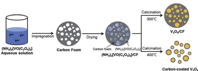
Fig. 12 Schematic of the preparation of carbon-fabricated V<sub>2</sub>O<sub>5</sub> samples (CF300 and CF400).<sup>117</sup>
