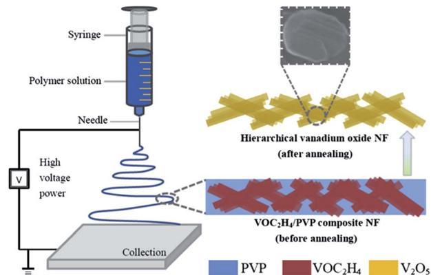
Fig. 6 Schematic showing the strategy for fabricating hierarchical  $V_2O_5$  nanofibers.<sup>79</sup>
