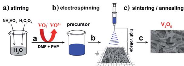
Fig. 3 Electrospinning reaction process for  $V_2O_5$  micro/nanorods.<sup>54</sup>
