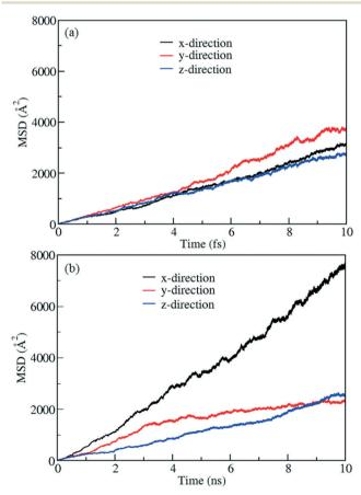
Fig. 9 MSD profiles for methane in methane filled CR0-CR0p substituted IRMOF-7-Cl2 (a) without E-field and (b) with E-field (2 V
