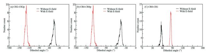
Fig. 8 Rotational dihedral angle distributions of (a) CR2-CR2p (b) CR0-CR0p and (c) CR0-CR1 substituted IRMOF-7-Cl<sub>2</sub> structures at 300 K under
