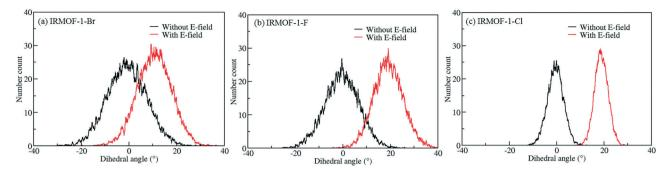
Fig. 2 Distribution of the rotational dihedral angle of the ligands in (a) IRMOF-1-Br, (b) IRMOF-1-F and (c) IRMOF-1-Cl at 100 K with and without E-field (8 V nm<sup>-1</sup>).
