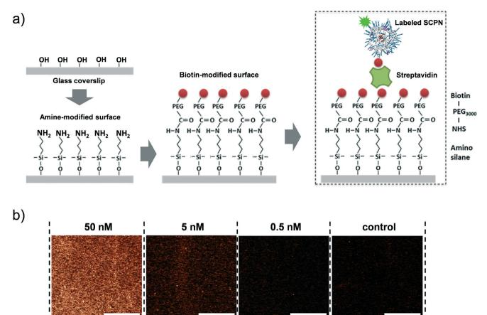
Fig. 6 Surface immobilization of biotinylated SCPNs. a) Experimental design. b) Confocal images showing biotinylated and Alexa Fluor® 488labeled SCPN on a functionalized coverslip. The images show SCPNs immobilized in various concentrations and a corresponding control measurement where no SCPNs were added. The bar represents 40 and 4 µm in the top and bottom panel, respectively.
