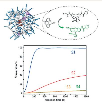
Fig. 4 Carbamate cleavage reaction of S1-S4 catalyzed by P1@Cu(i) ([P1] = 2 μM, [CuSO<sub>4</sub>] = 10 μM, NaAsc = 1 mM, substrate = 30 μM). The kinetic curves were recorded via fluorescence spectroscopy (ex. 495 nm; recorded at 520 nm) followed with normalization according to the conversions obtained from LC-MS.
