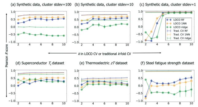
Fig. 3 Pearson R vs. k in k-fold CV (traditional CV) or k-means clustering (LOCO CV) across our benchmark datasets and several ML methods. Error bars represent the sample standard deviation of R across 10 CV runs at each value of k.
