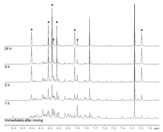
Fig. 3 NMR spectrum (400 MHz, CDCl<sub>3</sub>) between 7.0 and 8.7 ppm of the reaction of TFB + rac-CHDA immediately after mixing, and after 1, 2, 4, and 24 hours. Asterisks indicate peaks arising from CC3-RS and CC3-SR, confirmed by 2D NMR, MS, and analysis of pure cage sample (ESI† section 2); daggers indicate peaks assigned to CC3-R- or -S.
