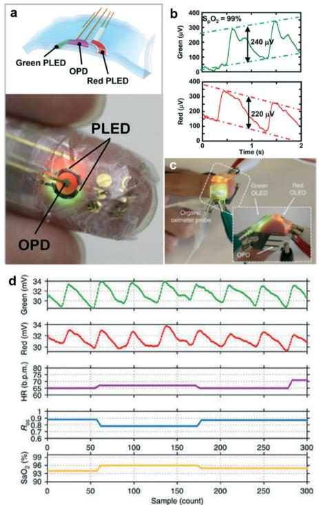
Fig. 14 Reflectance based layout and application picture of the pulse oximeter system with concentric LED's and circular photodiode scheme (a), with resulting signal output (b). Organic transmission based oximeter (c) with resulting raw data and signal extraction (d).
