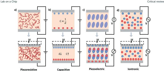
Fig. 5 Schematics illustrating the different modalities of mechanical sensors. a) Piezoresistivity; b) capacitance; c) piezoelectricity; <sup>190</sup> d) iontronic.
