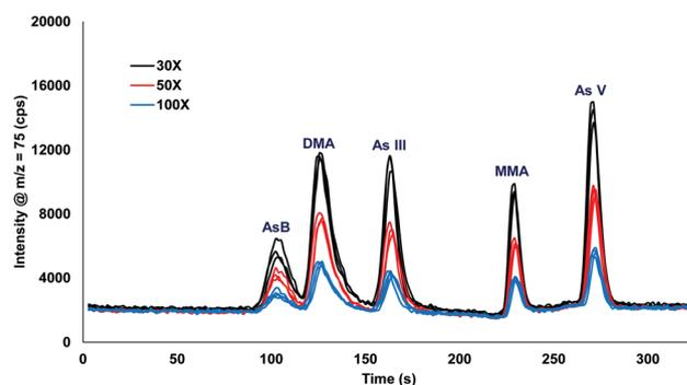
Fig. 3 Inline dilution (30X, 50X, and 100X dilution factors) of urine samples spiked with 10 ppb arsenic species.
