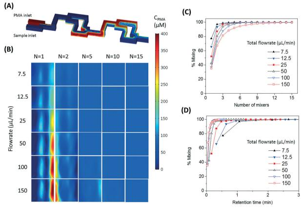
Fig. 2 (A) Demonstration of SAR mixing mechanism: simulated cross-sectional concentration of inlets and the first two mixers at a flowrate of 150 μL min<sup>-1</sup>. (B) Simulated PMA concentration profiles at cross sections after 1, 2, 5, 10, and 15 SAR mixers at flowrates ranging from 7.5 to 150 μL min<sup>-1</sup>. (C and D) Simulated percentage of mixing plotted over number of mixing units passed (C) and total retention time in the mixers (D).
