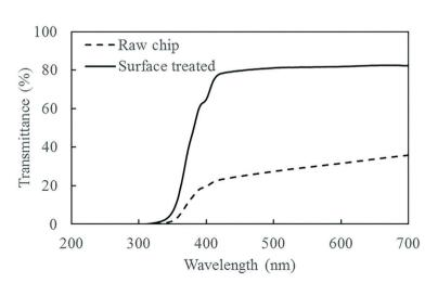
Fig. 3 (A) 3D printed channels at designed sizes of (from left to right) 500 μm, 400 μm, 300 μm, 200 μm, and 100 μm. (B) Light transmittance of the 3D printed chip, with and without rubbing mineral oil onto surface, over 200 to 700 nm wavelength range.
