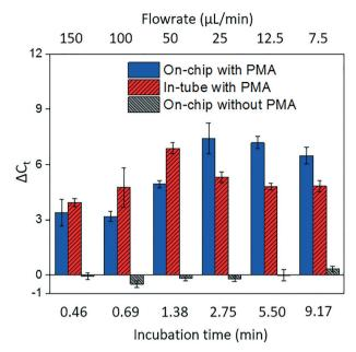
Fig. 4 The effectiveness of dead cell discrimination with PMA treatment. The experimental results were quantified by real-time PCR and expressed as the differences in the cycle number ( $\Delta C_t$ ) for samples before and after PMA pretreatment. The performance was tested under various flowrates, which corresponds to different light incubation time. The error bars represent the standard error (SE) of  $\Delta C_t$ .
