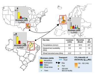
Fig. 3 Illustration of three potential BECCS value chain to a UK-based BECCS facility: using domestic pellets, which minimises transport distance, or importing pellets from Louisiana (USA) or Maranhao (Brazil). Factors such as carbon intensity of electricity, precipitation, biomass yield, marginal land area and wheat harvested area are paramount when determining BECCS optimal value chain.
