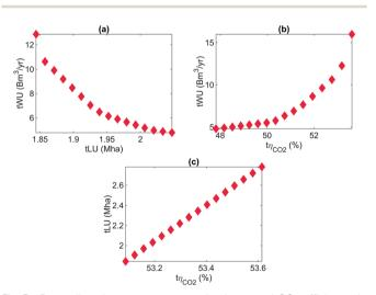
Fig. 5 Pareto lines between water use, land use, and  $CO_2$  efficiency, in the median scenario. There are strong trade-offs between water use and the other two objective functions. However, the trend of the pareto lines for these two relations ((a) and (b)) indicate the presence of tipping points which could reconcile the different objectives. CO2 efficiency decreases marginally when land use increases, showing the proximity of these two
