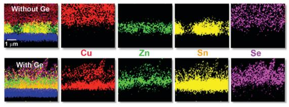
Fig. 2 Cross-sectional elemental distribution of samples with and without Ge (25 nm below the CTZ precursor) after reaching the first temperature plateau (t1) determined by EDX (Cu, Zn, Sn and Se. Mo is depicted in blue just in the overlapped mapping for guidance).
