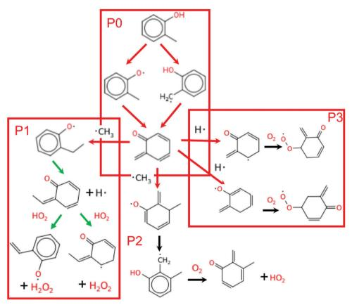
Fig. 8 The reaction pathways of o-cresol in the engine-like simulation just prior to final ignition: t = 46.2 ms and T = 925 K. Red arrows signify reactions that consume radicals, black arrows are radical neutral, and green arrows produce radicals.
