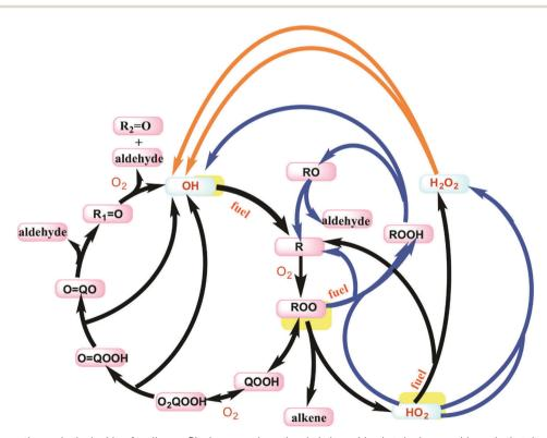
Fig. 4 Main reaction pathways in the ignition for alkanes. Black arrows show the chain branching ketohydroperoxide cycle that dominates below 690 K. Blue arrows show various heat-generating reactions for 690 K < T < 800 K. The orange arrows show the decomposition of H<sub>2</sub>O<sub>2</sub> to OH radicals which predominantly occurs above 800 K.
