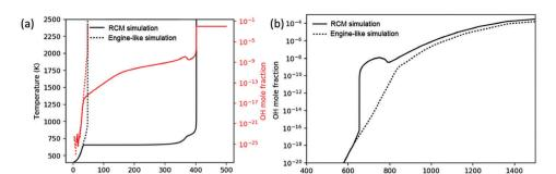
Fig. 5 (a) Temperature and OH mole fraction profile of rapid compression machine (RCM) and engine-like simulations. (b) OH mole fraction concentration as a function of temperature in RCM and engine-like simulations.
