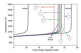
The predicted temperature history of the engine-like simulations using different fuel blends. PRF90: 90% iso-octane/n-heptane; PRF100: pure iso-octane; pure *n*-butane; 2% additive/*n*-butane. Conditions:  $\phi = 1$ ,  $T_0 = 400 \text{ K}$ ,  $P_0 = 1.09 \text{ bar}$ , adiabatic, effective V(t) defined by RON100 P(t).
