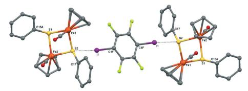
Fig. 4 Crystal structure diagram of 2, showing its I–S halogen-bonded trimolecular assemblies ( $[CpFe(CO)(\mu_2-SPh)]_2$ )<sub>2</sub>( $\mu_2-DITFB$ ). Hydrogen atoms are omitted for clarity. Selected distances (Å): I(1)–S(2), 3.130(1). Selected angles (°): C(1F)–I(1)–S(2), 173.9(1); Fe(1)–S(2)–I(1), 111.91(4); I(1)–S(2)–C(17), 102.5(1); I(1)–S(2)–Fe(2), 118.86(4). Dotted lines link S and I atoms at a distance shorter than the sum of the S–I vdW radii. 18
