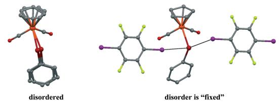
Fig. 3 The disorder of CpFe(CO)<sub>2</sub>TePh molecules in a parent crystal (LADWOE<sup>19</sup>) is "fixed" by two p-DITFB molecules in cocrystal 1.
