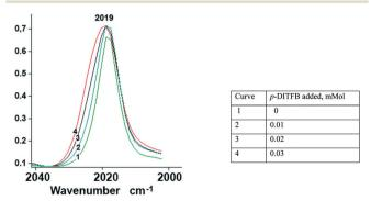
Fig. 1 Unsymmetrical hypsochromic broadening (ca.  $\sim$ 4 cm<sup>-1</sup> half-width) of the  $\nu$ (CO) band at 2019 cm<sup>-1</sup> as a result of gradual addition of p-DITFB to a 0.025 mmol cyclohexane solution of CpFe(CO)<sub>2</sub>TePh.
