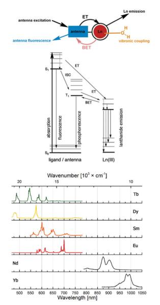
Fig. 1 Antenna effect, with major deactivation pathways shown in colour, and productive pathways for lanthanide sensitization in black (top). Emission spectra of the most commonly used lanthanide(III) emitters (bottom).
