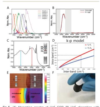
Fig. 5 (A) Absorption spectra of HgS CQD (B) HgS absorption with oleylamine and atomic ligand (C)  $1S_e - 1P_e$  and  $1P_e - 1D_e$  absorption spectrum (D) intraband and bandgap correlation-based k·p model (E) IR microscope image of doping controlled HgS permission from ref. 24. Copyright 2016 American Chemical Society. (F) Flexible HgSe CQD film.
