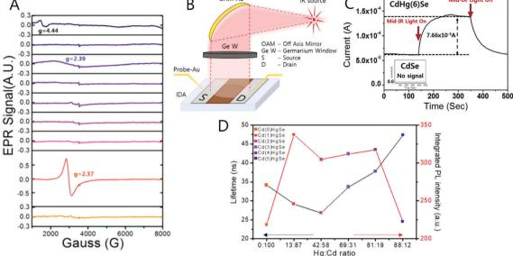
Fig. 9 (A) EPR spectra of CdHgSe series measured in room temperature (B) the schematic photocurrent measurement setup and (C) photocurrent response and (D) lifetime and photoluminescence relation. Adapted with permission from ref. 63. Copyright 2017 American Chemical Society.
