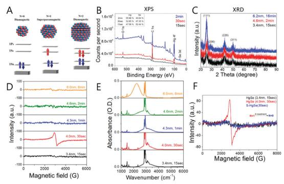
Fig. 6 (A) Schematic diagram of electron occupation of conduction band (B) XPS and (C) XRD data of HqSe (D) EPR signal and (E) absorption spectra of HgSe (F) the EPR signal of HgSe before (red), after (blue) and as synthesized (black). Adapted with permission from ref. 40. Copyright 2017 American Chemical Society
