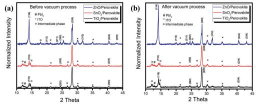
Fig. 2 X-ray diffraction patterns of perovskite films deposited on ZnO,  $SnO_2$  and  $TiO_x$  substrates: (a) before vacuum-processing and (b) after vacuum-processing. The XRD patterns are all normalized by the (220) peaks located at 28.3°.
