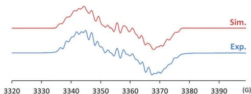
**Fig. 2** Experimental (bottom) and simulated (top) EPR spectra of **2** ( $g = 2.0107$ ; hyperfine coupling constants:  $a(^{14}\text{N}) = 23.4, 9.1, 6.9 \text{ MHz}$ ,  $a(^{11}\text{B}) = 6.7 \text{ MHz}$ ,  $a(^1\text{H}) = 5.3, 3.6 \text{ MHz}$ ,  $a(^{19}\text{F}) = 2.6, 1.7 \text{ MHz}$ ).
