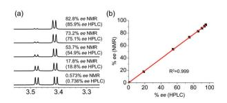
Fig. 6 (a) Partial  $^1$ H NMR spectra showing the methyl peaks of 1-phenylbutanol (3, 10 mM) with various enantiomeric excess in the presence of a CASA (10 mM) in CD $_3$ CN and (b) a linear plot between the % ee values determined by HPLC and NMR.
