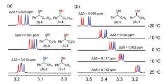
Fig. 3 The effect of (a) hydrophobicity and (b) temperature for chiral solvation of hydroxyl groups of alcohols with CASA-Na in CD3CN.
